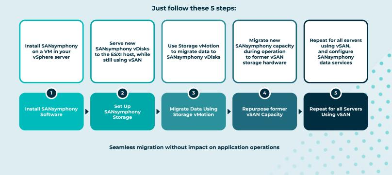
Please note that the first step requires having sufficient storage capacity available provisionally. This can easily be achieved by temporarily attaching capacity from JBODs, any direct attached storage (DAS), SAN capacity, or even from vSAN itself. Of course, this capacity is not needed after the transition took place, so it can be repurposed or simply returned.
