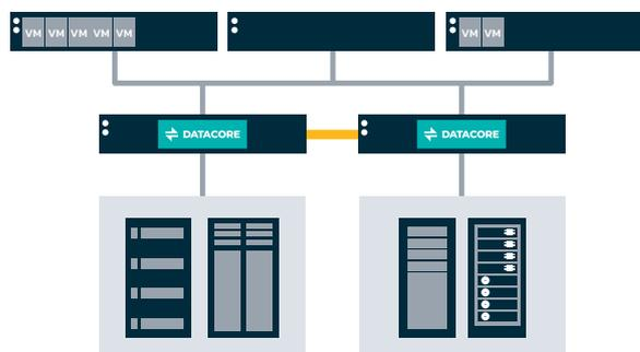
2 nodes. If one node experiences a failure, the second node will continue to host production IO without causing any downtime to core business applications. This type of protection is like an insurance policy that pays off whenever a SAN array fails.
